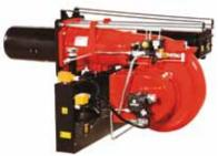
Burners for heavy oil at two stages, fan at high pressurisation, combustion head with adjustment at high efficiency and high flame stability, hydraulic system of regulation combustive air on the two stages of flame.
