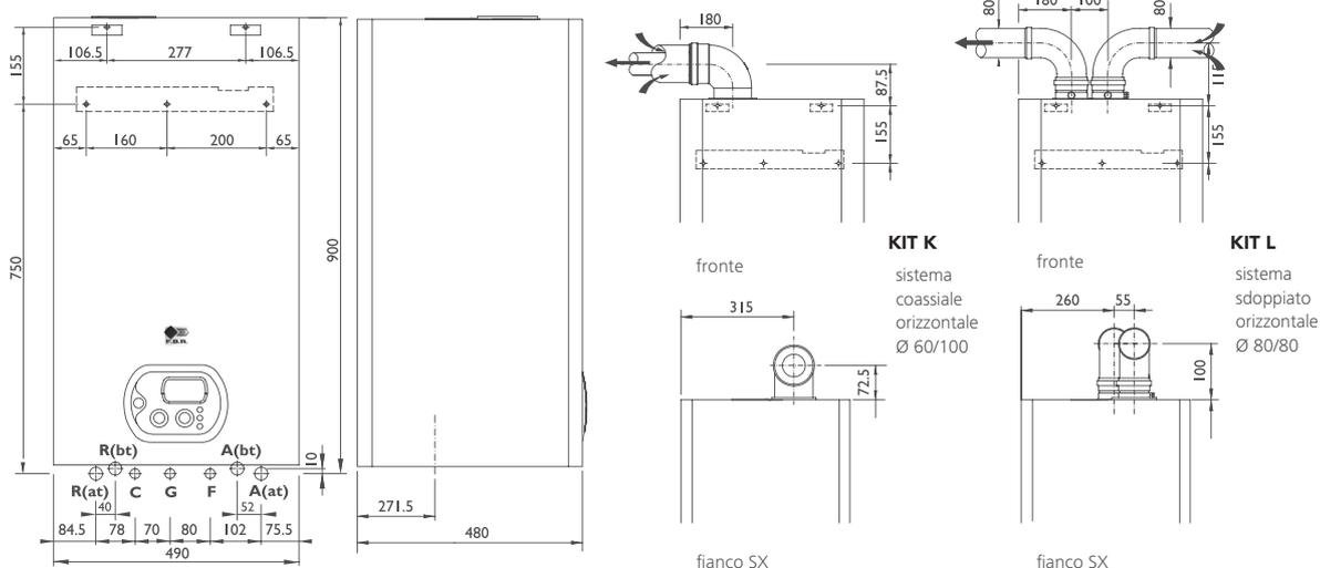
**A(at)** Andata Ø 3/4" - **A(bt)** Andata Ø 3/4" - **R(at)** Ritorno Ø 3/4" - **R(bt)** Ritorno Ø 3/4" - **C** Calda Ø 1/2" - **F** Fredda Ø 1/2" - **G** Gas Ø 1/2" - **SC** Scarico condensa Ø 25
